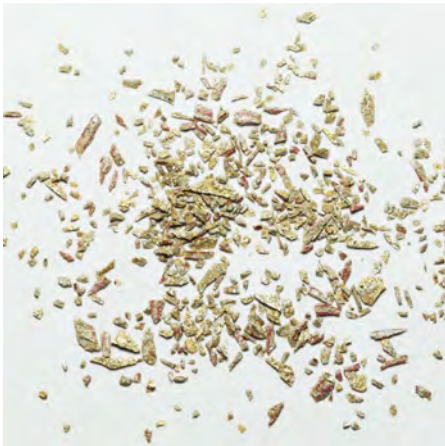
(c) Enamel flakes remaining in the sift.
