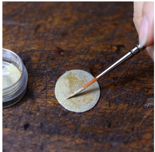
Figure 10: Application of a thin layer of enamel, everywhere.
