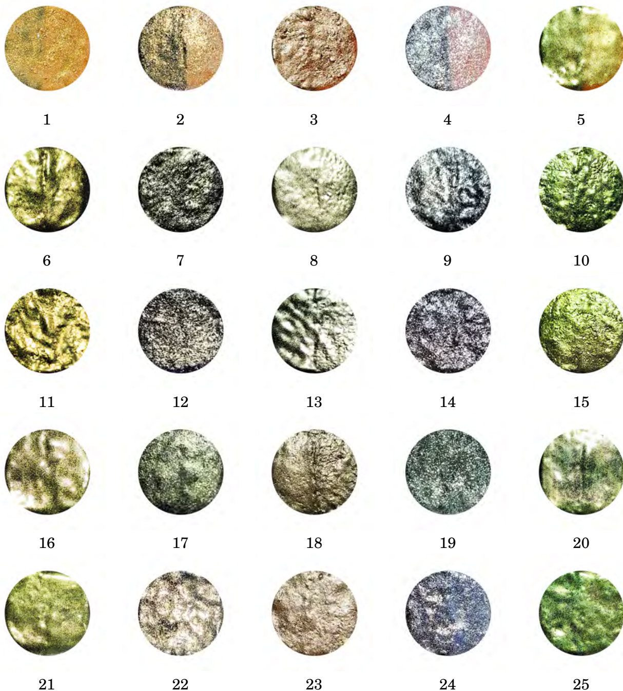
Figure 2: On the left side, the color is applied over the black base. On the right side, the color is applied on copper. The undertone is not clearly visible. Consult Figure 4) to find out the undertones of individual enamels.
