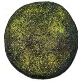
(a) 35 sec at 810 °C — Sugar firing.
