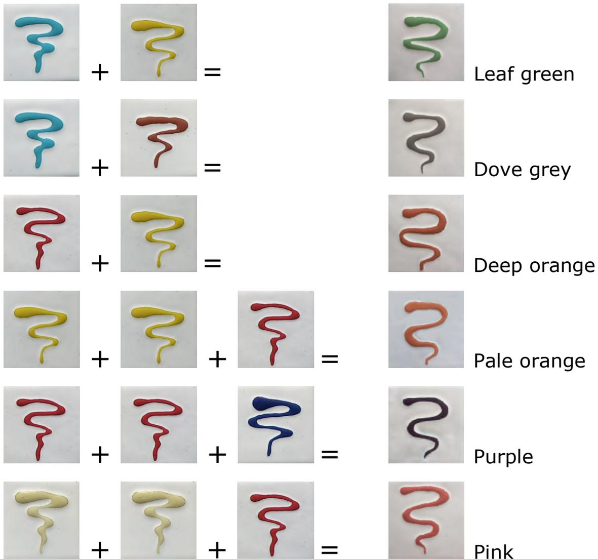
Sample images fired on copper with a base layer of 263T6/50 white enamel powder
