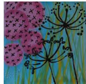
Samples of the enamel pens fired onto steel with ground coat and a base of titanium white. On the image to the right the pens have been used along with pink and blue powdered enamel.
