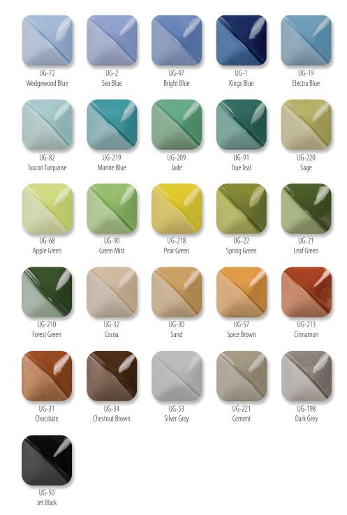
Chips shown represent Fundamentals® Underglaze applied to low-fire earthenware greenware, then fired to cone 04 bisque. S-2101 Clear was applied to the right-side of the chip and fired to cone 06.
