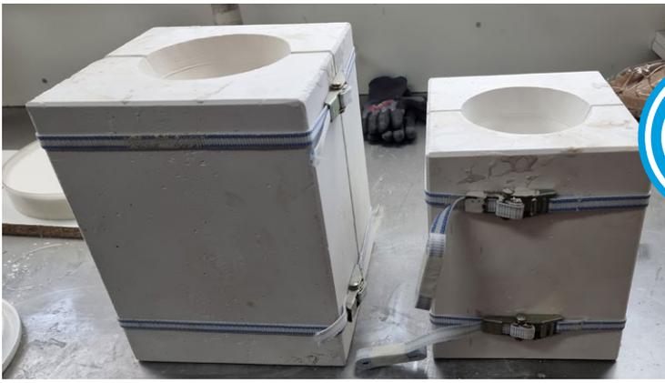
In this example we have casted vases with stoneware casting slip. The casting,- setting,- and drying time before the firing are all dependent on:
